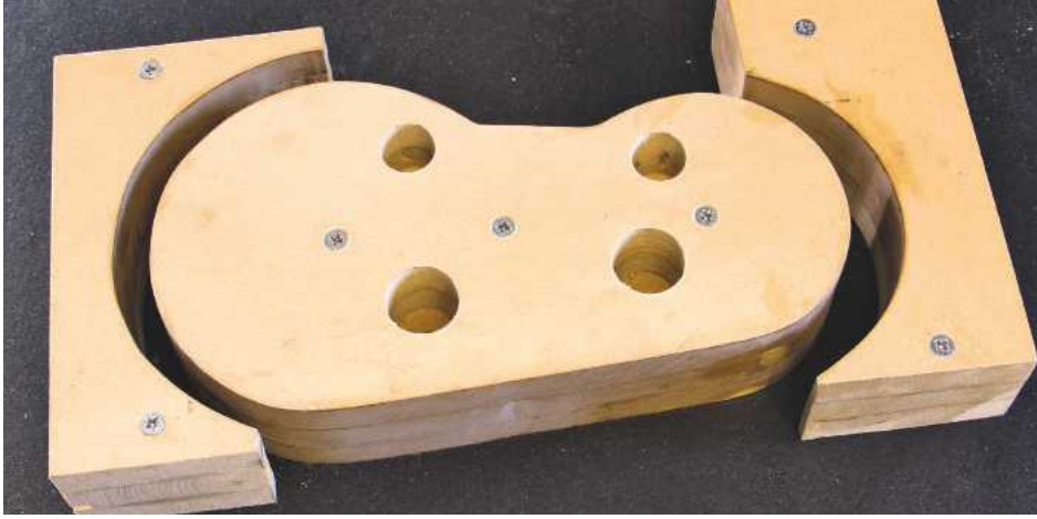
To experiment with laminating to create curved shapes, Dave built a former from MDF...
